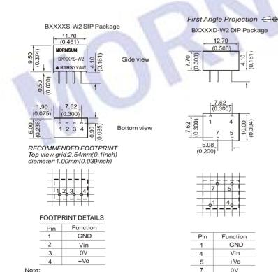
Note: Unit:mm(inch) Pin diameter:0.50mm(0.020inch) Pin diameter tolerances: $\pm 0.10$ mm( $\pm 0.004$ inch)
