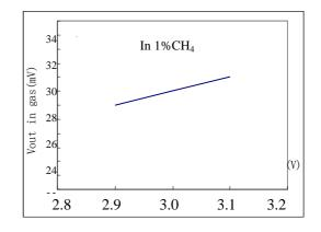
The drift in air per year is less than  $\pm 2$ mV, in 1%CH<sub>4</sub> is less than  $\pm 2$ mV. For a short period storage (in 2 weeks), the sensor need 30mins 'preheating to stabilize. for more than one year storage, it need more than 5 hours peheating.
