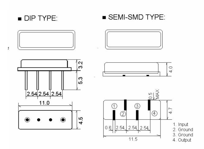
■Recommended layout of PCB(MM) (Tolerance ± 0.2MM)
