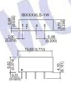
RECOMMENDED FOOTPRINT Top view,grid:2.54\*2.54mm(0.1\*0.1inch), diameter:1.00mm(0.039inch)
