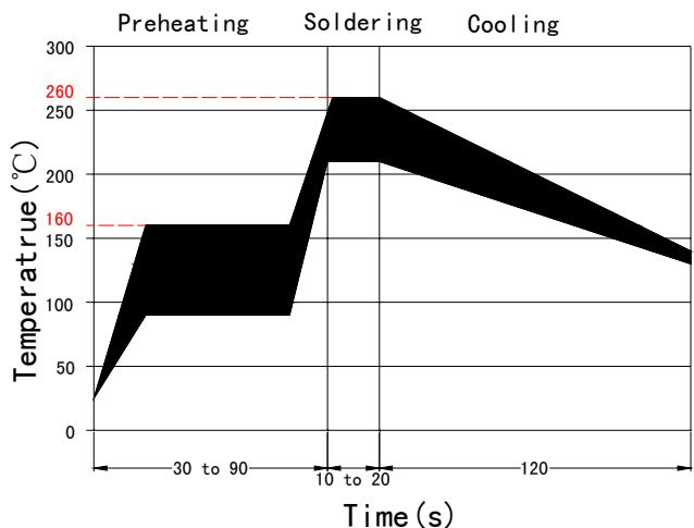
\* Recommended reflow methods: IR, Vapor phase oven, hot air oven, wave solder.
