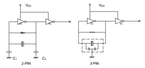
$\begin{array}{lll} \text{IC:} & & \text{TC74HCU04} \\ V_{\text{DD}}\text{:} & & +5\text{V} \pm 0.1\text{V} \\ \text{R:} & & 1\text{M}\Omega \\ \text{C_1, C_2:} & 30\text{PF} \end{array}$
