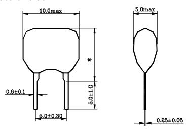
\*:13.01-23.99MHz,10.0max; 24.00-31.99MHz, 7.5max; 32.00-50.00MHz, 6.5max.
